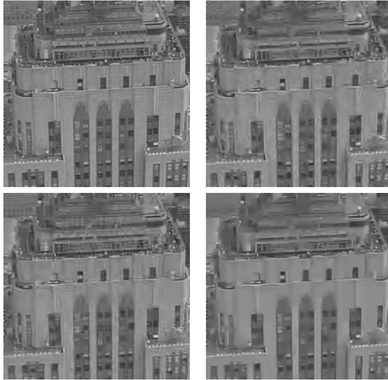
Fig. 7. 256 \times 256 portion at (480,416) of the City image coded at 0.17bpp. Clockwise: original image; coded by JPEG 2000; coded by H.264-JM; coded by the proposed adaptive block transform with pre/post-filtering.
